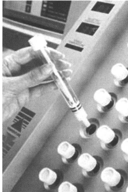
Figure 7.2b An impedance measurement cell being placed into the instrument.
