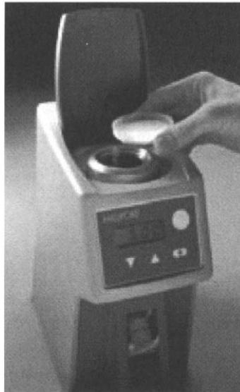
Figure 6.12 Placing the membrane in the AutoSpray station.
